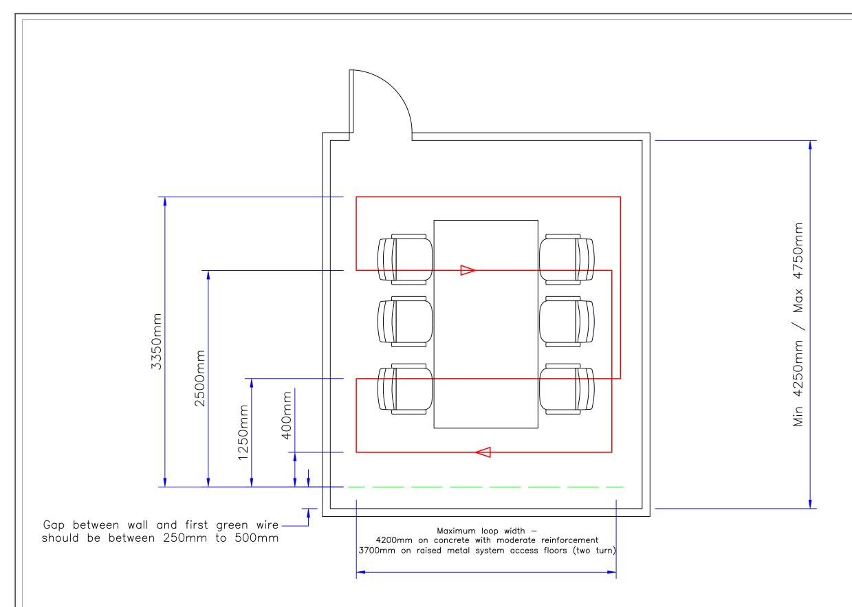
This design is intended for rooms with a Y dimension between 4.25m and 4.75m, the gap at the top and bottom of each array should be increased or descreased accordingly to keep the loop dimensions exactly as shown.
