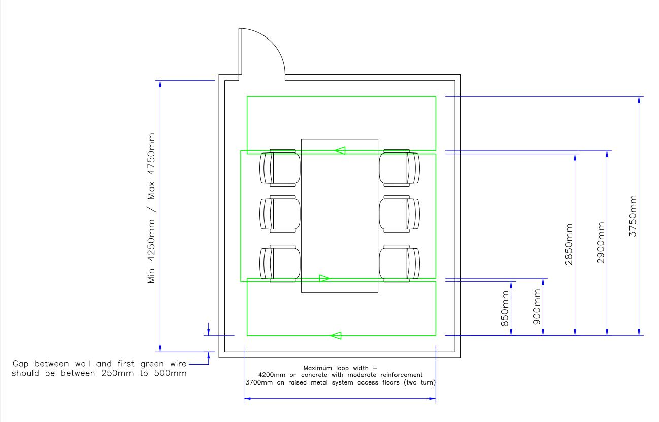
This design is intended for rooms with a Y dimension between 4.25m and 4.75m, the gap at the top and bottom of each array should be increased or descreased accordingly to keep the loop dimensions exactly as shown.
